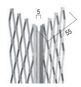
Corner profile made of aluzinced steel, for surface plaster in interior areas, sharp-tipped head. Use profiles in accordance with data sheet Planning and Application of Metallic Plaster Profiles.
