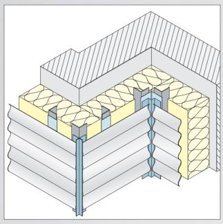
Corner profiles for inside corners form a clean, precise facade cladding stop.
