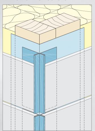
When aluminium corner profiles are used, the vertical profile should may correspond with a joint of the facade cladding. The general use of joint tapes can prevent water from penetrating.
