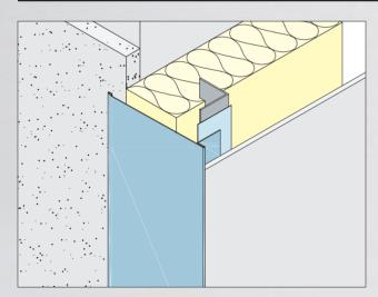
The connecting profiles connect the facade cladding and the different surfaces of the facade, such as the plaster, and thus facilitate a simple and precise transition. They fully cover and protect the cutting edges of the facade boards and cover the substructure on the side.
