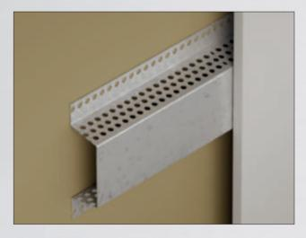
The PROTEKTOR Omega ventilation profile (Art.-Nr. 9363) is a hat profile made of aluminium with ventilation holes. The height of the profile is 30 mm; the base is 60 mm wide. Ventilation holes with a diameter of 5 mm are placed along the profile. The free ventilation cross-section at the 30 mm leg is 75 cm²/running metre. The material thickness is 1 mm.The Protektor Omega ventilation profile is versatile.
