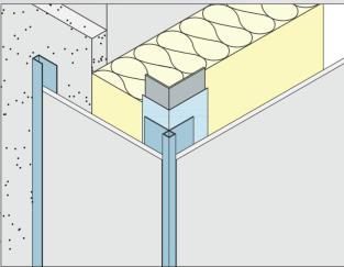
The connection of a curtain wall via a corner to another surface, for example a plastered surface or ETICS, can easily be carried out with an edge profile and a U-edge profile. For example, here with edge profile no. 9440 and U-edge profile no. 9450. Protektor has a large selection of façade profiles.
