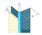
Corner profile made of aluzinved steel, for thin-layer plaster of 5 mm and thicker in interior areas.
