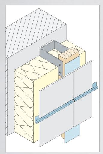
The joint profiles or h-profiles made of aluminium or PVC are used for horizontal joints. They reduce the penetration of moisture. Please ensure that the boards are not placed directly on the profile but that a joint of approx. 5 to 10 mm remains as indicated by the facade cladding manufacturer.
