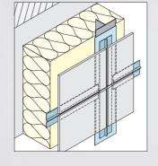
The aluminium joint profile or corrugated profile subtly depicts the joint whilst effectively closing it. The beading along the profile also centres and guides the facade cladding joint. The profiles are therefore available in widths of 6 mm and 9 mm for different joint widths. The corrugated profile may be used horizontally or vertically.
