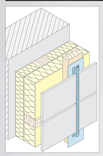
The joint profiles made of aluminium or PVC are used for vertical joints. Ensure that the facade cladding has room for expansion depending on the particular application. The aluminium joint profiles and top hat profiles can be installed on the front or the rearside of the facade cladding.
