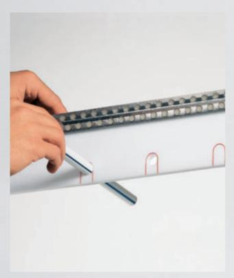
Exact pipe openings can be produced by puncturing the foam strip with a piece of pipe. Then cut through the foam strip with a straight cut downwards.
