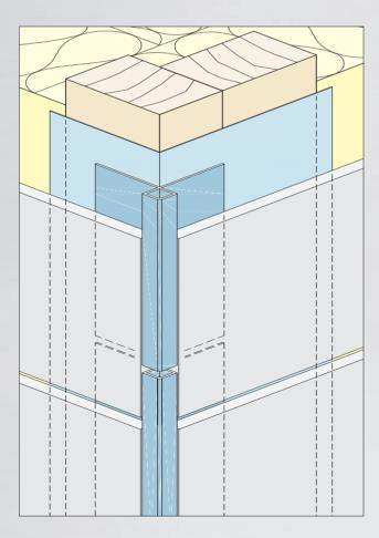
The vertical profile joints of the aluminium corner profiles can also be offset with the joint of the facade cladding. The general use of joint tapes can prevent water from penetrating.
