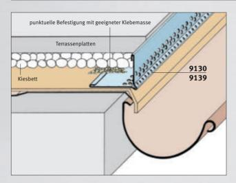
The gravel trap strip is ideally suited for loosely laid large balcony and terrace plates. Use suitable adhesive cement for securing gravel trap strip point by point. A suitable, load-bearing surface and superstructure must be installed as a substrate for the balcony and terrace plates. Suitable gravel/grit is to be appropriately compressed. The gravel trap strip is not to be strained by loads or movement caused by the balcony and terrace plates.
