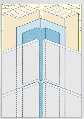
When aluminium corner profiles are used, the vertical profile should may correspond with a joint of the facade cladding. The general use of joint tapes can prevent water from penetrating.
