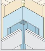
Corner profiles are used for facade design. They fully cover and protect the cutting edges of the facade boards and thus form a clean, precise edge.
