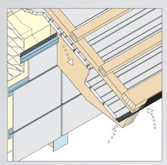
The ventilation profiles 9056 and 9059 are used in the upper facade area and under the window sills. The profiles can be used for board thicknesses of 4 to 6 mm and 8 to 15 mm.
